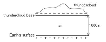
The lower plate of the capacitor is the Earth's surface and the upper plate is the base of the thundercloud.
