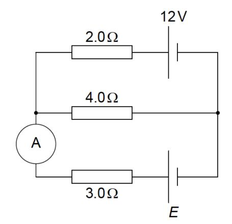
The top cell has electromotive force (emf) 12V. The emf of the lower cell is unknown. The ideal ammeter reads zero current. Calculate the emf E of the lower cell.
