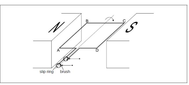
The ends of the coil are connected to slip rings and brushes. The plane of the coil is shown at the instant when it is parallel to the magnetic field. Only one coil is shown for clarity.
