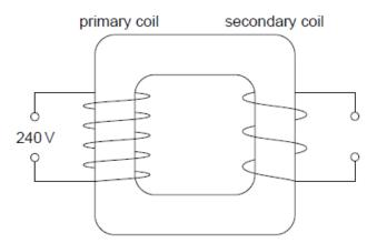
The number of turns in the primary coil is 1800 and that in the secondary coil is 90.
