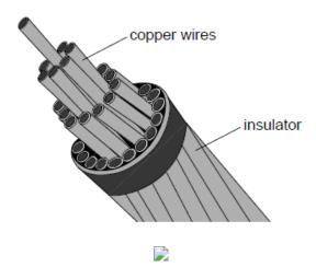
The cable consists of 32 copper wires each of length 35 km. Each wire has a resistance of 64  $\Omega$ . The cable is connected to the ac generator which has an output power of 110 MW when the peak potential difference is 150 kV. The resistivity of copper is 1.7 x 10<sup>-8</sup>  $\Omega$  m.
