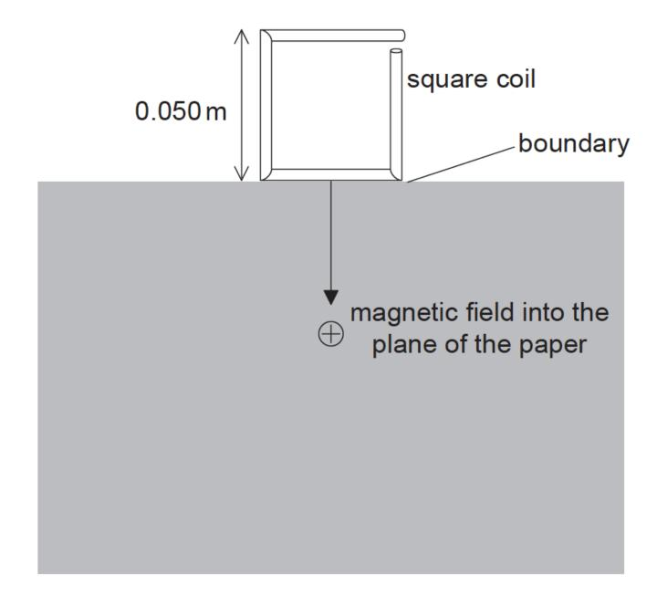
Each side of the coil is 0.050 m long. The dimensions of the magnetic field region are greater than that of the coil. The magnetic field strength is 25 mT.
