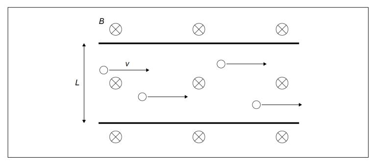
(i) Show that the potential difference V that is established across the conductor is given by V=vBL.
