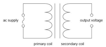
The transformer has 100 turns in the primary coil and 1200 turns in the secondary coil. The peak value of the voltage of the ac supply is 220 V. Determine the root mean square (rms) value of the output voltage.
