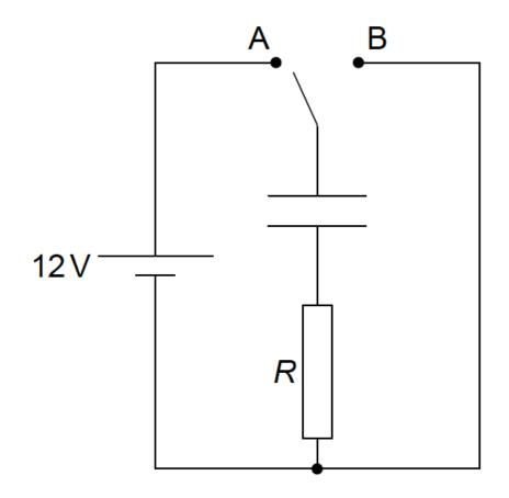
At t=0 the switch is placed at position A. The graph shows the variation with time t of the voltage V across the capacitor. The capacitor has capacitance  $4.5\mu$ F in a vacuum.
